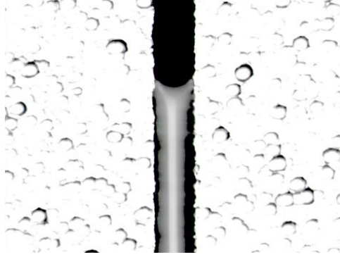
Figure 5. A 50:50 vol.:vol. MeOH:H 2 O mixture in a micro-machined capillary slot having a width w of 140 \mu\text{m} and a height h of 230 \mu\text{m} ( R = 1.64 ).
