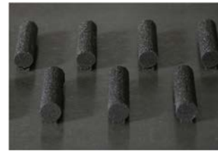
Fig. 9. Small cermet electrodes manufactured by the powder bed additive process.
