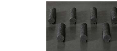
Fig. 9. Small cermet electrodes manufactured by the powder bed additive process.
