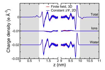
FIG. 3: Charge density within the electrode and the electrolyte for a finite field of  $0.1 \text{ V nm}^{-1}$  or the corresponding applied potential of 1.1 V. The contributions of water molecules and ions to the total charge distribution are also shown; they were shifted by  $-0.01 \text{ e Å}^{-3}$  for a better readability. The grey-shaded areas correspond to the electrodes (the CCS was translated in order to match with the ECS setup).
