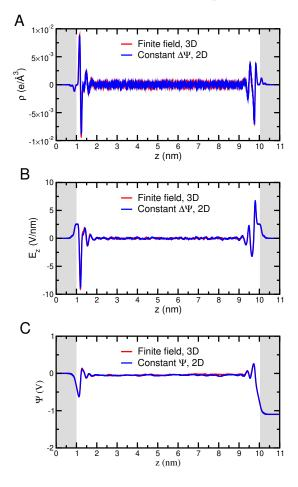
FIG. 4: Charge density (A), electric field (B) and Poisson potential (C) profile for an applied field of 0.1V/nm (corresponding to a potential drop across the cell of 1.1 V. The gray-shaded area corresponds to the electrodes (the CCS was translated in order to match with the ECS setup).
