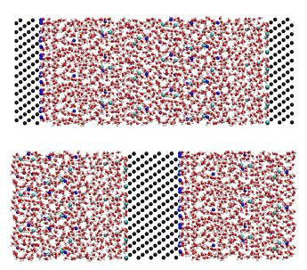
FIG. 1: Top: electrolyte-centered supercell (2D PBCs), with fixed applied potential between two electrodes ( $\Delta\Psi=\Psi_{\rm right}-\Psi_{\rm left}$ ). Bottom: conductor-centered supercell (3D PBCs), with a finite field **E** and a single electrode in which the potential of the atoms is set to the same value  $\Psi_{\rm electrode}$ .
