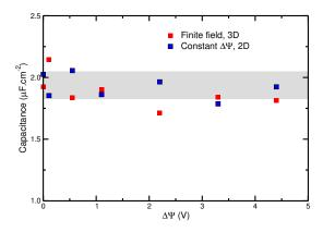
FIG. 7: Capacitance obtained using the fluctuationdissipation theorem for the finite electric field (red) and constant potential (blue). The grey-shaded area corresponds to the confidence interval obtained through the  $Q(\Delta\Psi)$  relation
