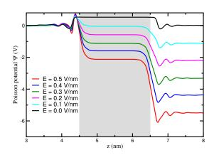
FIG. 6: Poisson potential profile for the single electrode under an applied electric field (corresponding to potential drop across the cell of 0 to  $5.5~\rm V$ ). The gray-shaded area corresponds to the electrode.
