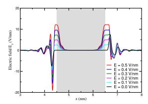
FIG. 5: Electric field profile for the single electrode under an applied electric field (corresponding to potential drop across the cell of 0 to  $5.5~\rm V$ ). The gray-shaded area corresponds to the electrode.
