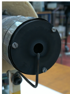
Figure 2. External tungsten igniter.
