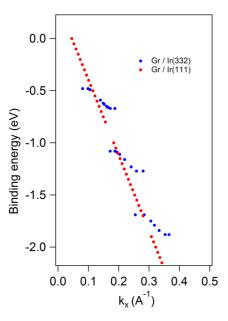
FIG. 6. Comparison between gap openings due to moiré and a one-dimensional periodicity. Simulation of gap openings in the one-dimensional periodicity of Fig. 2(a) (blue) and on the moiré of a Ir(111) surface (red). The minigaps due to Ir(111) moiré do not correspond to the gaps by nanostructuration as they appear at different k locations.
