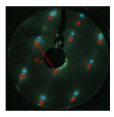
FIG. 3. LEED pattern of Ir(332) at 148 eV showing the  $G_{1\times 1}$  vector of the Ir(111) substrate and the G vector due to the facet periodicity. This G vector allows us to determine the spatial periodicity. In this case it is  $L=1.8\pm0.2$  nm along the  $\lceil \overline{121} \rceil$  direction.
