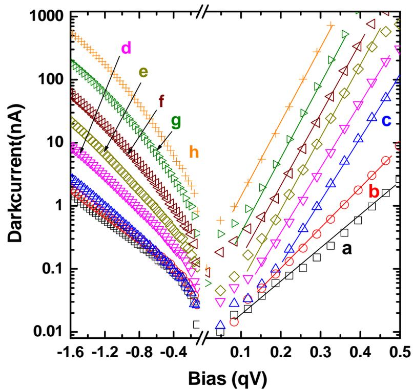
Fig. 3 : Tunnel photocurrent versus bias, defined as the additional tunnel current under light excitation. For (a)  $I_{\text{set}} = -2500$ , (b)  $-2000$ , and (c)  $-1000$ , the dependence at reverse (negative) bias is exponential. Progressive departure from purely exponential behavior occurs for (d)  $I_{\text{set}} = 0$ , (e) 500, (f) 1500, (g) 2000 and (h) 3000.
