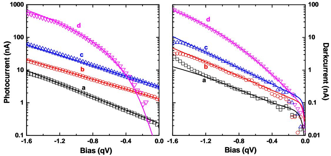
Fig. 8: Tunnel photocurrents from surface states and from the valence band calculated for  $I_{\text{set}} = -2500$  using Eq. (19) and Eq. (20) respectively. The other fixed parameter values that have been used are shown in Table 2. None of these currents is able to account for the data.
