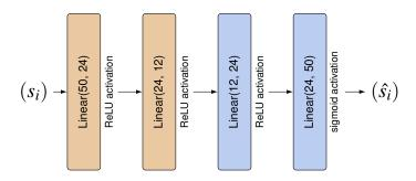
Fig. 6. Neural network architecture with two layers of progressive compression (encoding) and two layers of decompression (decoding).
