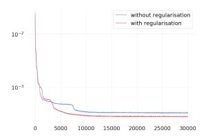
Fig. 7. Convergence of the MSE loss is at first slower but soon becomes better with regularisation (cluster 4,  $\lambda=10^{-2}$ ): final value for the MSE loss after 30,000 iterations is  $2.79\cdot 10^{-4}$  with regularisation but  $2.98\cdot 10^{-4}$  without.
