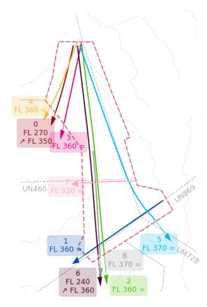
Fig. 5. The clustering method applied to our dataset trimmed to LFBBPT sector resulted in the nine following clusters. The altitude below the identifier of the cluster reflects the altitude profile of the centroid.
