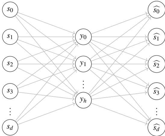
Fig. 3. Autoencoder neural network architecture with one layer
