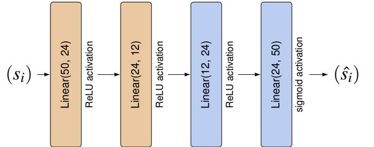
Fig. 6. Neural network architecture with two layers of progressive compression (encoding) and two layers of decompression (decoding).
