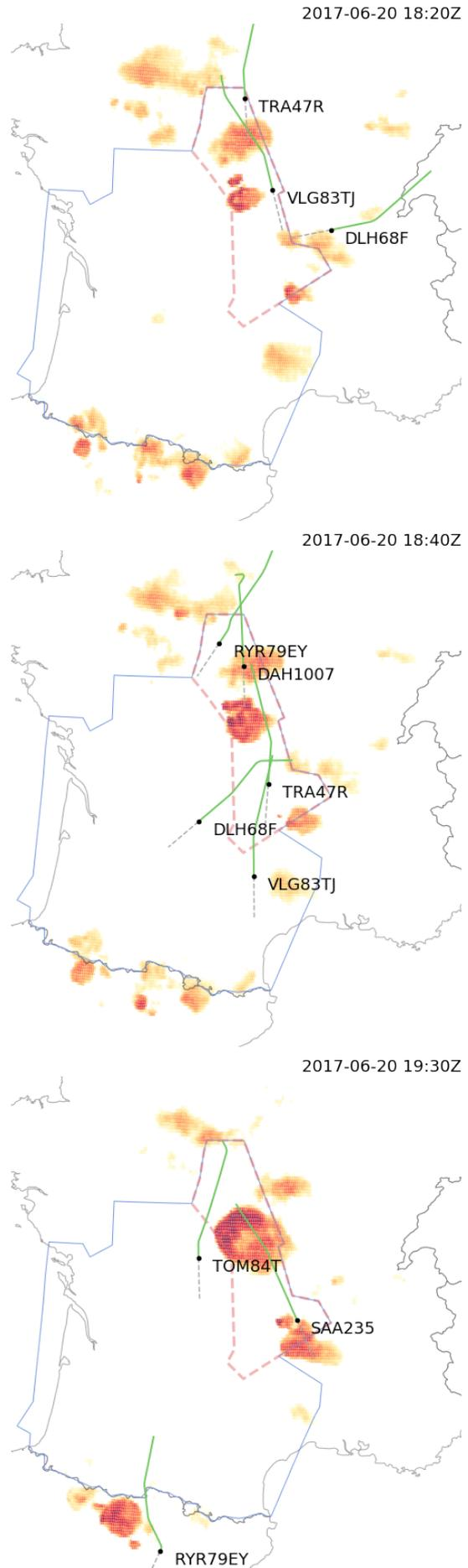
Fig. 14. Trajectories of aircraft flying to avoid cumulonimbus
