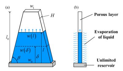
**FIG. 1.** Schematic illustration of capillary penetration incorporating evaporation effect in a trapezoidal porous plate: (a) oblique view; (b) side view.
