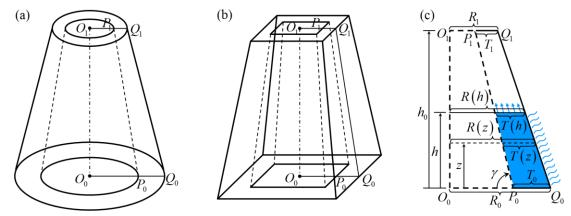
**FIG. 8.** Schematic illustration of 3D porous structures: (a) hollow circular frustum, (b) hollow square frustum, and (c) Intermediate cross-section of the 3D porous structures with capillary penetration incorporating evaporation effect.
