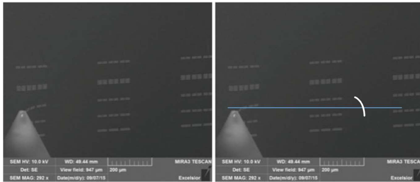
Fig. 24.15 Principle of alignment of probe tips with the patterns
