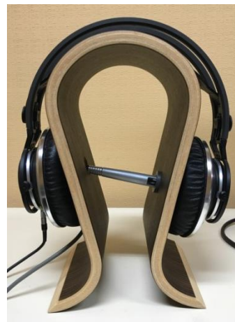
Figure 2. Illustration of the AKG K812 headset on its holder with the microphone to evaluate its frequency response.
