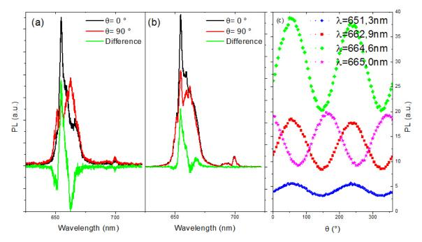
**Figure 1.** (a-b) Spectrum for two orthogonal polarizations (red and black) and the difference between them (green) for two different NPs of the same batch NR07. (c) PL intensity versus polarization for different wavelengths.
