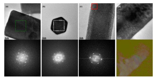
**Figure 6.** (a-c) HRTEM of NPs with below the FFT of the indicate area (a) NR09 with a typical FFT orthogonal to the c-axis (b) NR13 with a typical FFT parallel to the c-axis (c) NR11 with a FFT characteristic from an hexagonal phase trough the c-axis but observed orthogonally to the c-axis. (d) HRTEM of a NR06 with various defects below same image filtered with false color.
