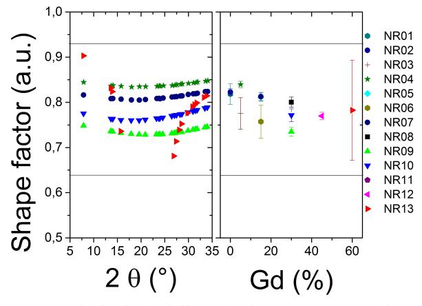
**Figure 4.** (a) Shape factor for each peak of four typical samples (NR04, NR07, NR09, NR10) and the most different sample (NR13) (b) Mean shape factor versus the expected gadolinium concentration
