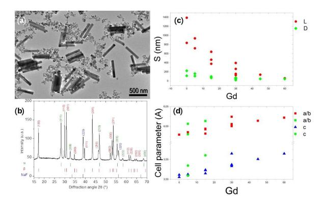
**Figure 3.**  $NaYF_4$  nanoparticles (a) TEM image with small cubes ( $\alpha$ -NaYF<sub>4</sub>) big nanorods ( $\beta$ -NaYF<sub>4</sub>) (b) typical X-Ray pattern of these particles (c) TEM NPs sizes S (L = lenght, D = diameter) and (d) cell parameter dependences vs Gd nominal doping with blue triangles and red squares for the main set of cell parameters of each batch and green stars and green circles for the second set of cell parameters
