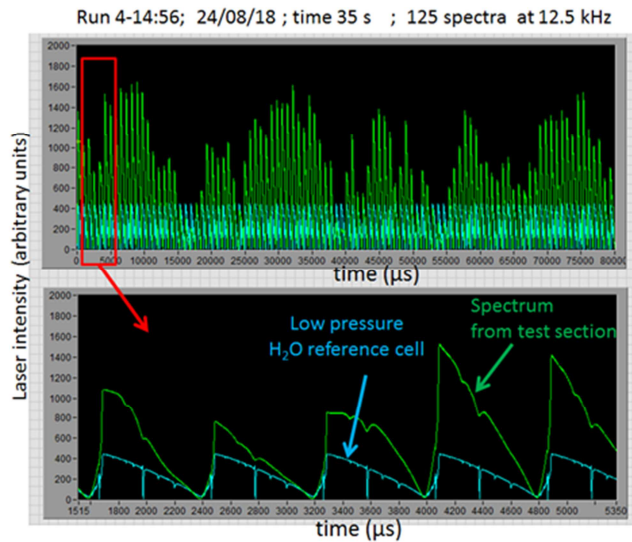
Fig. 6. One hundred successive spectra during a Mascotte run (taken at half run time).
