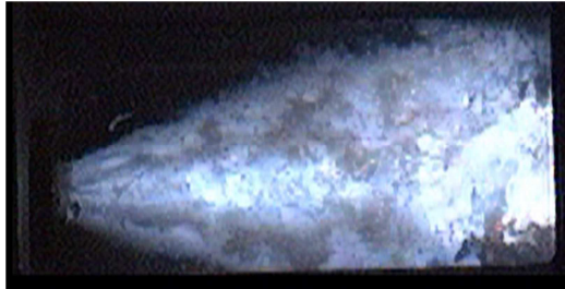
Fig. 1. Liquid oxygen / liquid methane flame produced by a single element coaxial injector.
