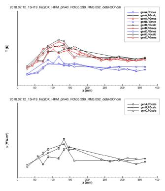
Fig. 7. Temperature and heat flux profiles for GOX injection. High mixture ratio (M=3.1) and moderate pressure (P=3.5 MPa) case.
