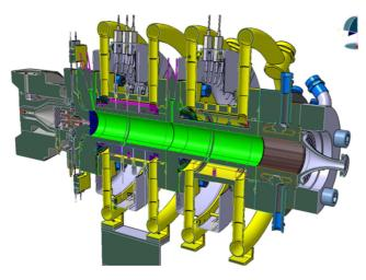
Fig. 1. The water-cooled BHM combustion chamber.
