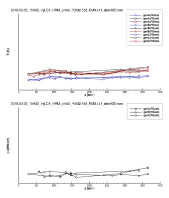
Fig. 6. Temperature and heat flux profiles for LOX injection. High mixture ratio case (M=3.4) and moderate pressure (P=3.3 MPa).
