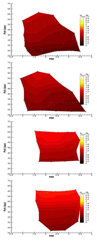
Fig. 9. Non dimensional heat flux maps for LOX injection in the (M, P) plane. Two lateral injectors positions and two injectors diameters in the following order LL 30, LL 40, LH 30, LH 40.
