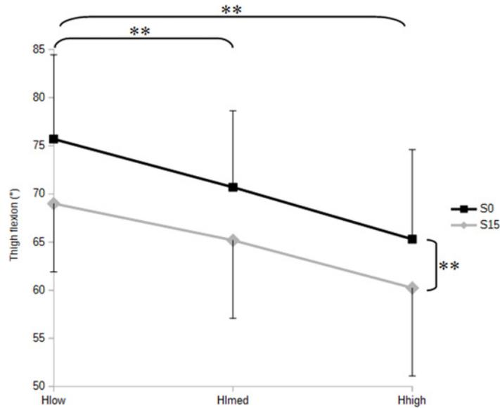
**Figure 5. Thigh flexion as a function of seat slope and height.** Mean values are illustrated in no sloping (S0) and 15° forward sloping (S15) conditions, with low (Hlow), medium (Hmed) and high (Hhigh) height settings. \*\* $p < 0.01$
