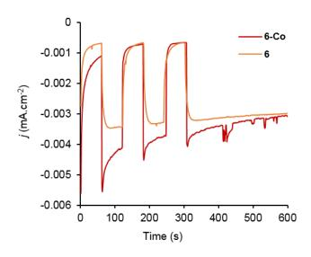
**Figure 6.** Chronoamperometric measurements under chopped-light using NiO electrodes sensitized with **6-Co** (red line) or **6** only (orange line) in acetate buffer (0.1 M, pH 4.5) at an applied potential of + 0.07 V vs. RHE (- 0.4 V vs. Ag/AgCl) under visible-light irradiation (400-800 nm, 65 mV.cm<sup>-2</sup>, 1 sun).
