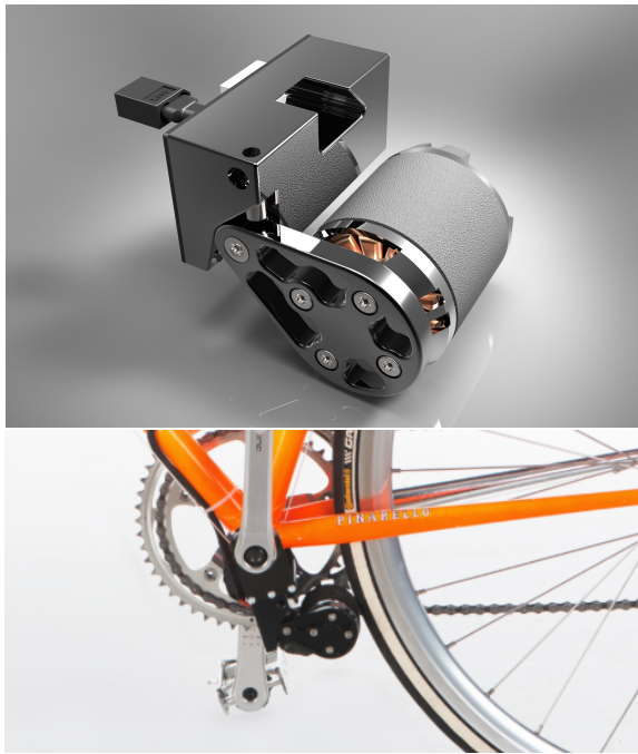
FIG. 2. Top: a ‘clip-on’ motor that turns a bike into an eBike; the bottom figure shows how the motor is fixed on the bike. Courtesy: add-e
