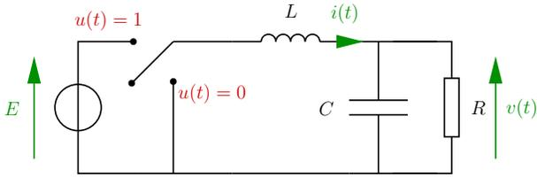
Fig. 2: Ideal representation of the buck converter
