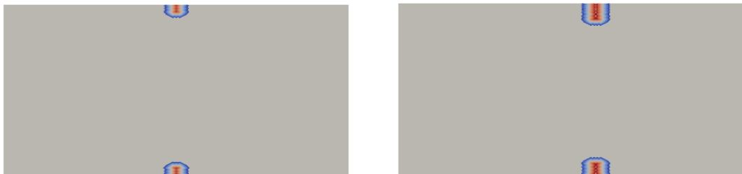
Figure 1: On the left, a channel configuration with an obstacle on the upper and lower walls. On the right, a channel configuration with a new obstacle at this time, translated with respect to the first one in the horizontal direction, and with a new length
