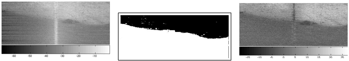
Fig. 2. Example of unsupervised BS (Backscattering Strength) compensation: from left to right, original BS map involving two seafloor types, segmentation map issued from the estimated posterior likelihood, compensated BS image.
