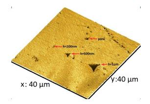
Fig. 16: An atomic resolution scanning probe microscopy image of a residual indent on a calcareous aggregate (natural) for different indentation depths h = 200, 500, 1000nm
