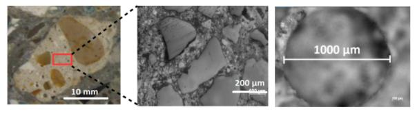
Recycle aggregate with a focus on the attached mortar
