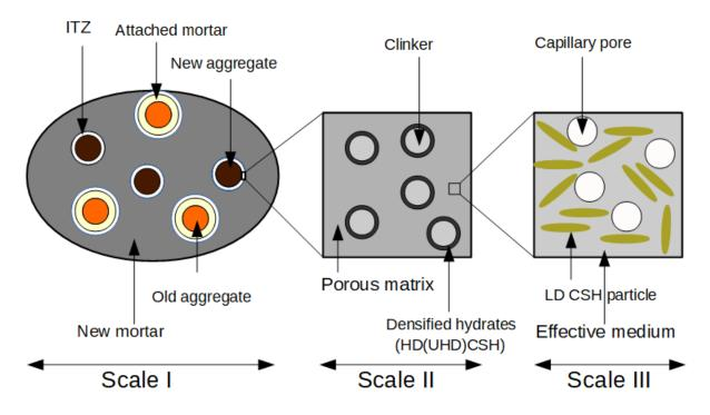
Fig. 28: Simplified representation of the microstructure of RAC
