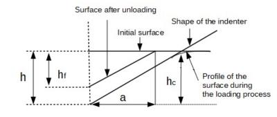
Fig. 10: Geometrical 2D representation of the contact area of Berkovich tip.
