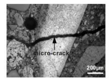
Fig. 8: Typical example of micro-crack observed in the attached mortar
