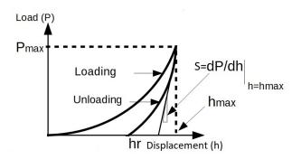
Fig. 9: Load and unloading profile
