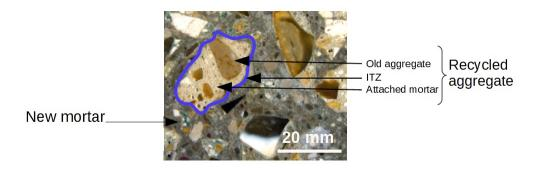
Fig. 1: Different phases in the microstructure of RAC
