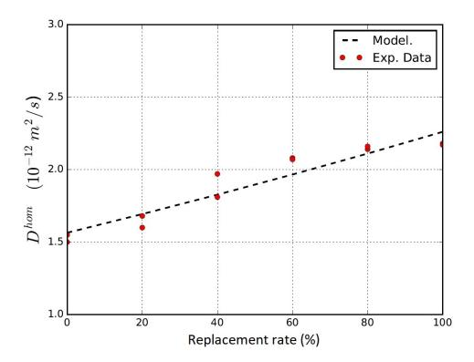
Fig. 30: Diffusion coefficient of RAC with different replacement rates (Obtained results for  $D_2 = 4.43 \times 10^{-12} m^2/s$ ,  $D_{\text{ITZ}} = 3.9 \times 10^{-11} m^2/s$ ).
