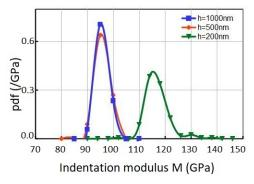
Fig. 19: Distribution (pdf) of the measured indentation modulus for siliceous aggregates
