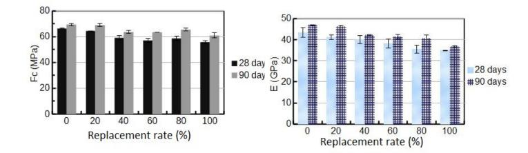
Fig. 2: Compressive strength for different replacement rates
