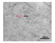
Fig. 14: Optical microscope image of the surface of calcareous aggregate (natural). Typical pore diameter is d = 100nm
