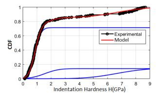
Fig. 27: Cumulative Distribution Function (CDF) of the indentation hardness (curves represented in blue are for individual phases)
