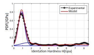
Fig. 26: Probability Density Function (PDF) of the indentation hardness (curves represented in blue are for individual phases)
