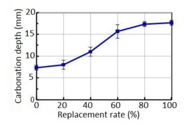
Fig. 5: Carbonation depth with different replacement rates
