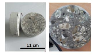
Fig. 20: Typical specimen submitted to micro indentation test
