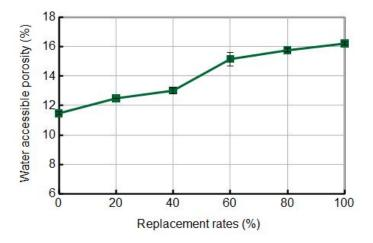
Fig. 4: Water accessible porosity with different replacement rates
