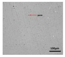
Fig. 15: Optical microscope image of the surface of siliceous aggregate (origin). Typical pore diameter is d = 100 nm
