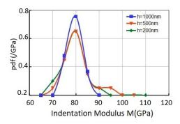
Fig. 18: Distribution (pdf) of the measured indentation modulus for calcareous aggregates
