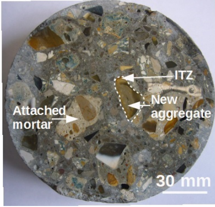
Fig. 11: Microstructure of a section of C[60] concrete with phases of interest.
