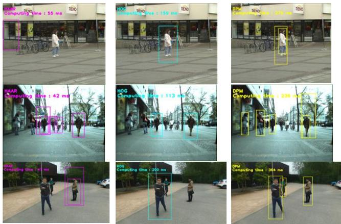
**Fig 1.** Comparison between HAAR (left), HOG (middle) and DPM (right) applied under three different datasets: TUD-Brussels (top row), ETH (middle row) with 640x480 image resolution, and ESIGELEC (bottom row) with 960x540 image resolution.
