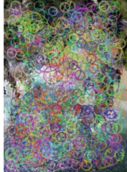
Figure 5. SURF points extracted from a sample image of the imageset under analysis
