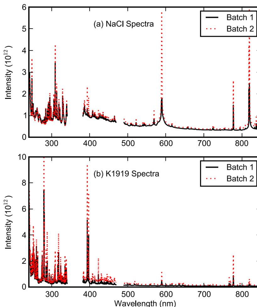
**Figure 8.** Comparison of (a) NaCl and (b) K1919 spectra collected in the first (solid black line) and second batches (dotted red line) of measurements at laser-to-sample distances of 1.6 and 3.0 m, respectively, after processing to correct for the geometric effects of distance.
