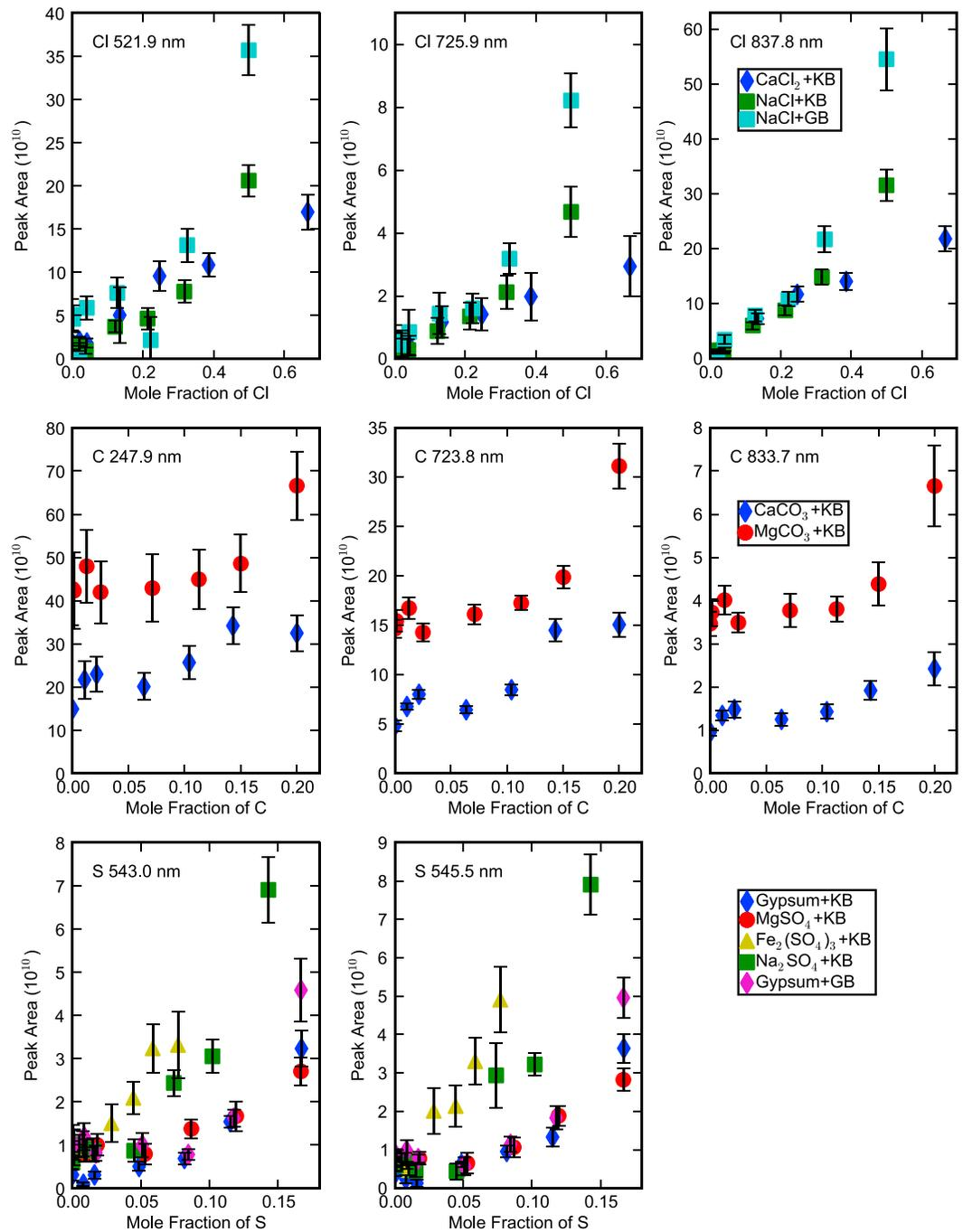
**Figure 5.** Calibration curves of peak area versus mole fraction of element for a selection of Cl, C, and S peaks and each salt + basalt combination (provided in the legend for each row). Peak areas are in units of photons/shot/mm<sup>2</sup>/sr. Calibration curves for remaining Cl and C lines are provided in Figures S3 and S4 in the supporting information.
