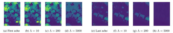
Fig. 1: Some rasters over residential area, for first echo (a-b-c-d) and last echo (e-f-g-h) with original rasters (a-e), SDAP filtering with  $\Lambda = 10$  (b-f),  $\Lambda = 200$  (c-g) and  $\Lambda = 5000$  (d-h). One can observe the interest of the last echo (second line) since structures below vegetation are clearly highlighted.
