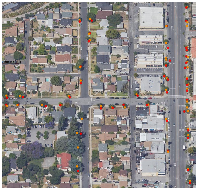
Figure 9. Small subset of tree predictions (red) overlaid to an aerial image (not used in our model) and compared to tree ground truth locations (orange).
