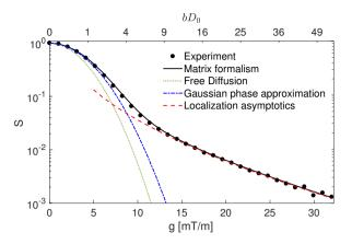
**Fig. 6:** Signal attenuation for diffusion inside phantom 2 (a cylinder of diameter 3.8 mm). Experimental results are shown by full circles and matrix formalism computation by a solid line. The signal for free diffusion is indicated by a dotted line, whereas the short-time approximation  $e^{-bD}$ , where D is given by Eq. (23), is plotted as a dashed-dotted line. The high-gradient asymptotic regime (25) appears as a dashed line.
