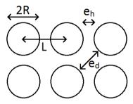
**Fig. 9:** Schematic representation of the rods showing the lengths  $e_{\rm d}$  and  $e_{\rm h}$ .
