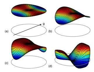
**Fig. 8:** Transverse magnetization computed by matrix formalism inside phantom 3 (a cylinder of diameter 2 mm) for four values of the gradient g: (a) 2 mT/m, (b) 5 mT/m, (c) 10 mT/m and (d) 32 mT/m. The direction of the gradient is indicated by an arrow.
