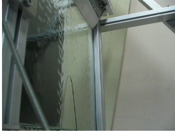
FIG. 22: Capillary waves in the liquid film around the dry patch (Rhodorsil 47V5 oil)
