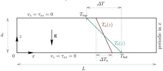
FIGURE 1. Rectangular, 2D, physical setup  $\Omega$ . The boundary conditions are periodic in the horizontal x direction. Stress-free, impermeable conditions apply on bottom and top boundaries, held at imposed hot  $T_{bot}$  and cold  $T_{top}$  temperatures.
