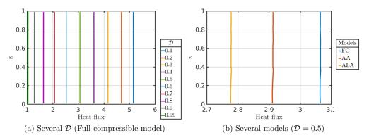
FIGURE 3. Heat flux profile along the vertical direction, averaged over the horizontal direction x and time, for r = 3 and  $Ra_{sa} = 10000$ .
