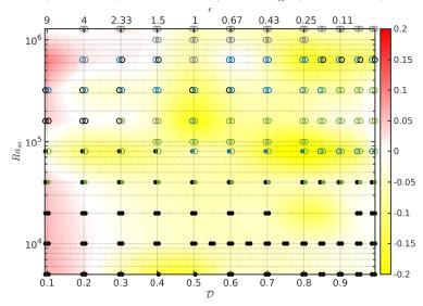
FIGURE 20. Relative difference of the ratio of the total viscous dissipation to the convective heat flux ((ratio<sup>FC</sup> – ratio<sup>ALA</sup>)/ratio<sup>FC</sup>) between the full compressible and anelastic liquid approximations, in the  $\mathcal{D}$ -Ra<sub>sa</sub> plane, for  $r=3, \gamma=1.4$ . The points (colored circles) follow the same code as in Fig. 14.
