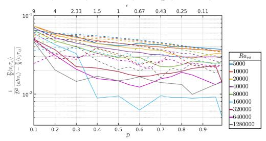
FIGURE 17. Relative weight of the shear-stress power contribution to the convected heat flux  $-\mathcal{D}/R \langle v_j \tau_{zj} \rangle / (\langle \rho h v_z \rangle - \mathcal{D}/R \langle v_j \tau_{zj} \rangle)$  divided by  $\mathcal{D}^2$  for the full compressible (solid lines) versus anelastic (dashed lines) calculations, for  $r=3, \gamma=1.4$  and a range of values of the superadiabatic Rayleigh number  $Ra_{sa}$ .
