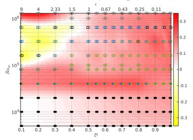
FIGURE 16. Relative difference  $\left(Nu_{sa}^{AA}-Nu_{sa}^{ALA}\right)/Nu_{sa}^{AA}$  of the superadiabatic Nusselt number  $Nu_{sa}=Q_{sa}/\Delta T_{sa}$  as a function of  $\mathcal D$  and  $Ra_{sa}$  between full anelastic AA and anelastic liquid ALA calculations, for  $r=3,\ \gamma=1.4$ . The points (colored circles) follow the same code as in Fig. 14, except they correspond now to the anelastic (AA, left symbols) and anelastic liquid (ALA, right symbols) numerical calculations.
