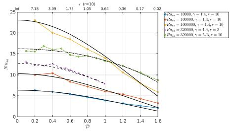
FIGURE 13. Superadiabatic Nusselt number  $Nu_{sa} = Q_{sa}/\Delta T_{sa}$  as a function of  $\mathcal{D}$  for the anelastic approximation with different values of  $\gamma$  and a range of values of the superadiabatic Rayleigh number  $Ra_{sa}$ . Black curves correspond to the analytic expression (8.16), using (8.7).
