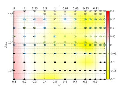
FIGURE 19. Relative difference of the ratio of the total viscous dissipation to the convective heat flux ((ratio<sup>FC</sup> – ratio<sup>AA</sup>)/ratio<sup>FC</sup>) between the full compressible model and the anelastic approximation, in the  $\mathcal{D}$ -Ra<sub>sa</sub> plane, for  $r=3, \gamma=1.4$ . The points (colored circles) follow the same code as in Fig. 14.
