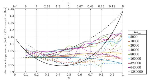
FIGURE 23. Ratio of the integral of viscous entropy sources,  $\mathcal{D}/R \langle (\dot{\epsilon}:\tau)/T_a \rangle$  (using the adiabatic temperature profile  $T_a$ ), to the convective heat flux divided by  $\mathcal{D}$  as a function of  $\mathcal{D}$  for the full compressible (solid lines) versus anelastic (dashed lines) calculations, for r=3,  $\gamma=1.4$  and a range of values of the superadiabatic Rayleigh number  $Ra_{sa}$ .
