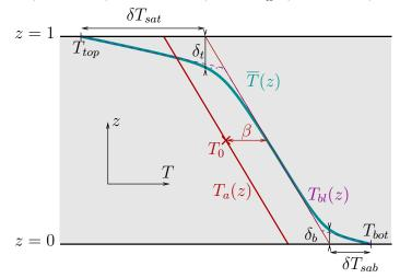
FIGURE 8. Typical horizontally-averaged temperature profile  $\overline{T}(z)$ , reference adiabatic profile  $T_a(z)$ , shifted adiabatic temperature profile  $T_a(z) + \beta$  and boundary layer amplitudes ( $\delta T_{sab}$  at the bottom,  $\delta T_{sat}$  at the top), and thicknesses ( $\delta_b$  at the bottom,  $\delta_t$  at the top). The dashed broken-line profile  $T_{bl}(z)$  is an idealized piecewise linear profile, with linear core and linear boundary layers.
