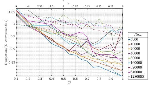
FIGURE 18. Ratio of the integral of viscous dissipation to the convective heat flux as a function of  $\mathcal{D}$  for the full compressible (solid lines) versus anelastic (dashed lines) calculations, for r=3,  $\gamma=1.4$  and a range of values of the superadiabatic Rayleigh number  $Ra_{sa}$ .
