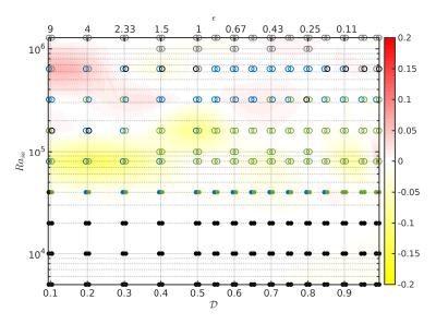
FIGURE 21. Relative difference of the ratio of the total viscous dissipation to the convective heat flux ((ratio<sup>AA</sup> – ratio<sup>ALA</sup>)/ratio<sup>AA</sup>) between the anelastic and anelastic liquid approximations, in the  $\mathcal{D}$ -Ra<sub>sa</sub> plane, for  $r=3, \gamma=1.4$ . The points (colored circles) follow the same code as in Fig. 14.
