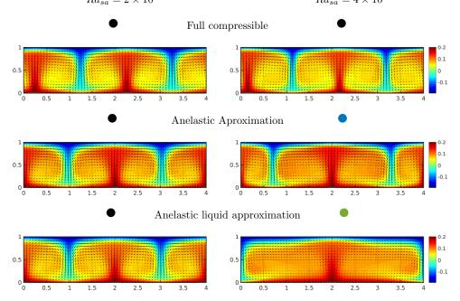
FIGURE 4. Comparison of the structure of the patterns of convection in full compressible FC, anelastic AA and anelastic liquid ALA approximations, for r = 3,  $\gamma = 1.4$  and  $\mathcal{D} = 0.6$  ( $\epsilon = 5/3$ ). Black dots indicate the presence of two symmetricals convective cells, blue dot two asymmetrical cells and green dot a single cell.
