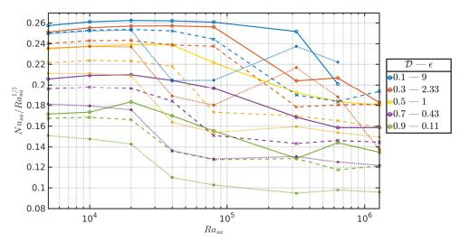
FIGURE 11. Superadiabatic Nusselt number  $Nu_{sa} = Q_{sa}/\Delta T_{sa}$ , divided by  $Ra_{sa}^{1/3}$ , as a function of  $Ra_{sa}$  for full compressible calculations (solid lines), anelastic approximation (dashed lines) and anelastic liquid approximation (dotted lines), for r = 3,  $\gamma = 1.4$  and a range of values of the dissipation number  $\mathcal{D}$ .
