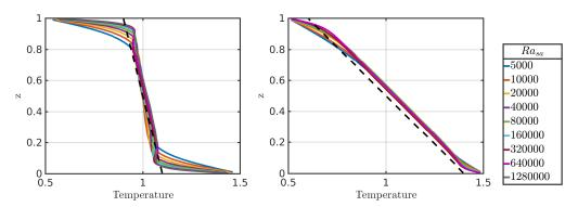
FIGURE 6. Average temperature profiles from the full compressible model FC, for  $\gamma = 1.4$  and a temperature ratio r = 3. The value of the dissipation number is  $\mathcal{D} = 0.2$  ( $\epsilon = 4$ ) on the left-hand side and  $\mathcal{D} = 0.8$  ( $\epsilon = 0.25$ ) on the right-hand side. The profiles are shown for various values of the superadiabatic Rayleigh number (reference adiabatic profile shown as dashed line).
