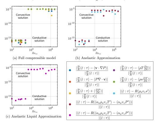
FIGURE 2. Computed differences between equivalent expressions for the viscous dissipation given by equation (5.2) for full-compressible solutions and by equations (5.3) and (5.4) for an elastic solutions, for r = 3,  $\gamma = 1.4$  and D = 0.8 ( $\epsilon = 0.25$ ).
