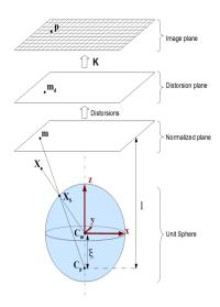
Fig. 3. Unified projection model.
