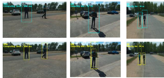
Figure 2. Comparison between HOG and DPM applied under ESIGELEC dataset (640x480-image resolution). Top row: HOG algorithm, Bottom row: DPM algorithm.
