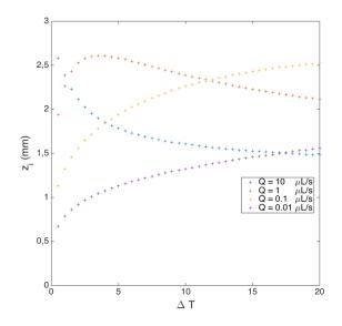
FIG. 10. Calculated height of the highest inflection point  $z_i$ , versus undercooling  $\Delta T$ , for distilled water. Other parameters are :  $\theta_0 = \pi/2$ ,  $R_0=1$  mm.
