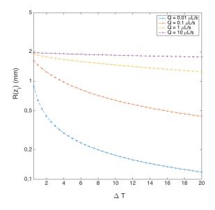
FIG. 12. Calculated radius of the frozen drop (distilled water) at  $z_i$ , versus undercooling  $\Delta T$ . Other parameters are :  $\theta_0 = \pi/2$ ,  $R_0=1$  mm.
