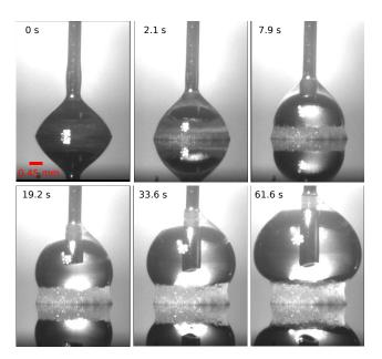
FIG. 2. Successive shapes of a drop of hexadecane freezing from its base on a cold substrate, under continuous feeding. Flow-rate  $Q = 0.1 \ \mu l/s$ ,  $\Delta T = 4^{\circ}$ . Under these conditions, the freezing drop adopts an overhanging shape, which constitutes its final one before the liquid on top collapses and falls under gravity.
