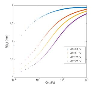
FIG. 11. Calculated radius of the frozen drop (distilled water) at  $z_i$ , versus flow rate, for different values of  $\Delta T$ . Other parameters are :  $\theta_0 = \pi/2$ ,  $R_0=1$  mm.
