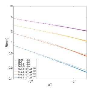
FIG. 7. Calculated radius of the frozen drop (distilled water) at a height of 2 mm versus undercooling  $\Delta T$ , for different flow-rates Q. Other parameters are :  $\theta_0 = \pi/2$ ,  $R_0=1$  mm.
