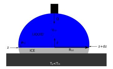
FIG. 3. Geometrical model for the solidification of droplet with continuous feeding rate Q. The liquid/solid interface is assumed to be flat, horizontal and the unfrozen liquid is assumed to adopt the shape of a spherical cap. Consequently, the axisymmetric shape is entirely defined by R(z), and the liquid drop forms an angle  $\theta(z) = \tan^{-1}(-\frac{dz}{dR})$  with the ice front.
