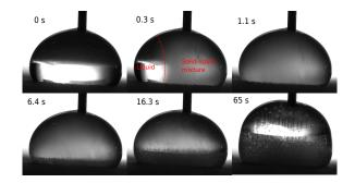
FIG. 13. Sequence of recalescence within a drop (snapshots 2 and 3), observed before the icewater front appears at much longer times. The initial time corresponds to the first image where recalescence appears. We note that the drop shape remains unchanged during recalescence.
