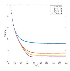
FIG. 8. Calculated radius of the frozen drop (distilled water) at a height of 2 mm versus  $(\pi - \theta_0)$ and different values of  $\Delta T$ . Other parameters are :  $Q = 0.1 \ \mu l/s$ ,  $R_0 = 1 \ mm$ .
