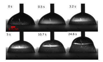
FIG. 1. Successive shapes of a drop of water freezing from its base on a cold substrate, under continuous feeding. After a first stage of fast spreading, the liquid is laterally pinned and reaches its final basal diameter. Then, the drop thickens and grows upwards as the freezing front progresses also upwards.
