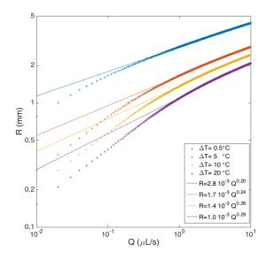
FIG. 6. Calculated radius of the frozen drop (distilled water) at a height of 2 mm versus flow rate for different values of  $\Delta T$ . Other parameters are :  $\theta_0 = \pi/2$ ,  $R_0=1$  mm.
