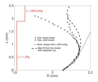
FIG. 14. Drop profile of liquid drop before (green) and after (blue) the solidification. Distilled water with initial contact angle  $\theta = 125^{\circ}$  and initial radius r = 2.15 mm.  $Q = 1.16 \ \mu l/s$ .
