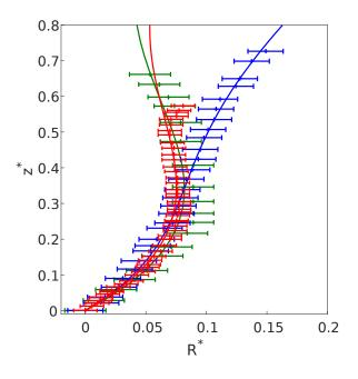
FIG. 5. Experimental and numerical shapes of frozen ice (water) drops for different flow-rate Q, with  $\Delta T=9$  °C and  $\theta =120^{\circ}$ . The data points (experiments) and related plain lines (numerics) correspond to :  $Q=0.16 \ \mu l/s$  (green)  $Q=0.32 \ \mu l/s$  (red) and  $Q=0.5 \ \mu l/s$  (blue)
