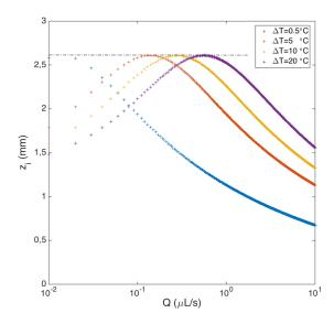
FIG. 9. Calculated height of the highest inflection point  $z_i$ , versus flow rate for the case of water and different values of  $\Delta T$ . Other parameters are :  $\theta_0 = \pi/2$ ,  $R_0=1$  mm.
