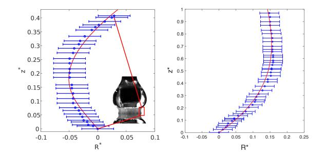
FIG. 4. Experimental and numerical shapes of a frozen drop. (a) Hexadecane with initial contact angle  $\theta_0 = 40^\circ$  and initial radius  $R_0 = 1.71$  mm.  $\Delta T = 4$  °C and  $Q=0.83 \ \mu l/s$  (b) Water with initial contact angle  $\theta_0 = 120^\circ$  and initial radius  $R_0 = 2$  mm.  $\Delta T = 9$  °C and  $Q=0.32 \ \mu l/s$
