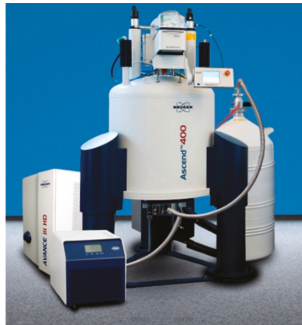
Figure 4. 400 MHz (9.4 T) NMR system of the Bruker company.
