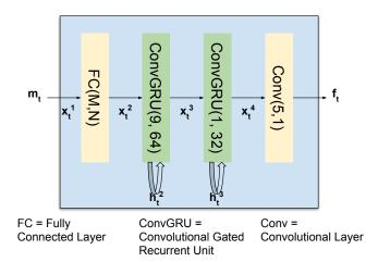
**Fig. 1**: Proposed recurrent neural network for single-pixel video reconstruction. The design is inspired by [10], but the convolutional layers are replaced by convolutional gated recurrent units (ConvGRUs) that maintain the long-term temporal dependency. ConvGRU $(K_s, F_m)$  designates a ConvGRU cell with convolutional kernels of size  $K_s \times K_s$  and  $F_m$  output feature maps.
