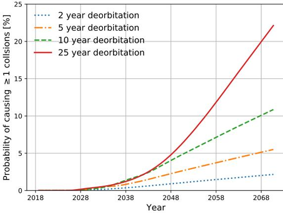
Figure 6: Probability of causing at least one collision for various de-orbitation scenarios: de-orbitation performed in 2 years, 5 years, 10 years, or 25 years. Constellation parameters are those specified in Table 2 .
