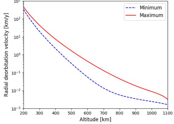
Figure 4: Radial drag velocity (pointing toward the Earth) as a function of the altitude for a spherical object of 2 m of diameter,  $1t/m^3$  of mass density, and a ballistic coefficient  $C_x$  equal to 3, for the minimum and maximum densities corresponding to the solar activity.
