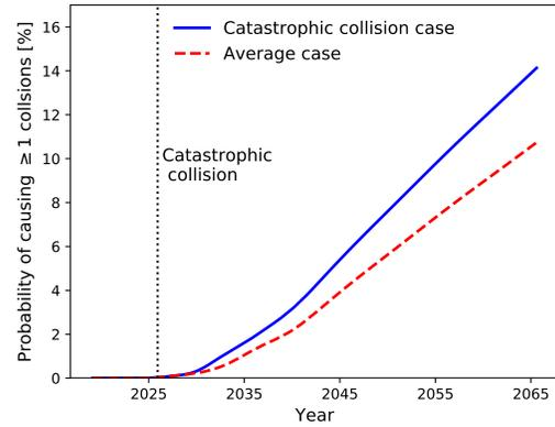
Figure 7: Probability for a de-orbiting satellite to be involved in a collision with a space debris, given that a catastrophic collision occurred in 2025, generating 3 000 objects larger than 10 cm.
