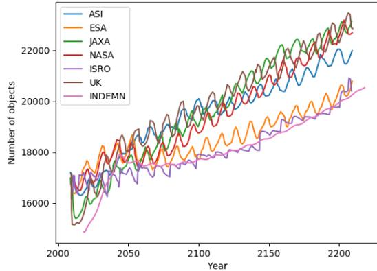
Figure B.8: Comparison of the simulation results by various codes developed by national and international agencies with the results provided by INDEMN for the IADC 12-08 benchmark.
