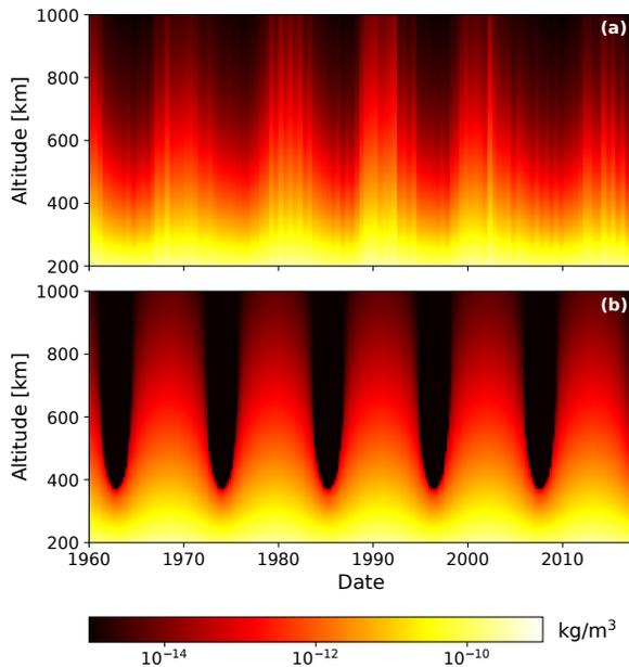
Figure 2: Comparison between the historical data retrieved from the NRLMSISE-00 Atmosphere model [14] averaged over orbital angles (a), and the fit proposed in Eq. 1) of this paper (b).
