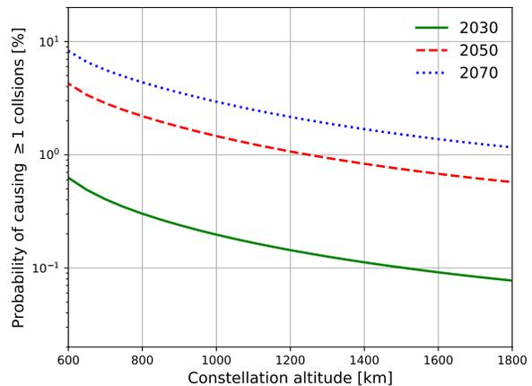
Figure 5: Risk for a de-orbiting satellite of the constellation to cause a collision as a function of the constellation altitude. The de-orbitation time is set to 2 years.
