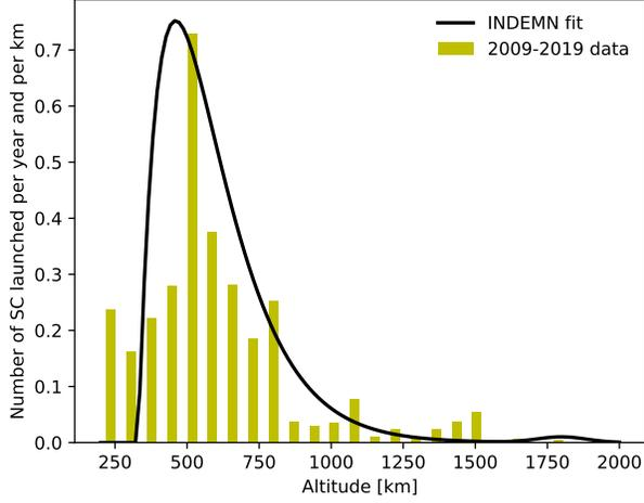
Figure 3: Spacecrafts launched per year and per altitude unit as a function of the altitude. The INDEMN fit is compared to historical data from spacetrack.
