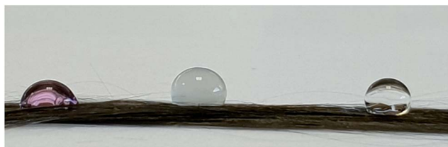
Fig. 6 Image showing the hydrophobic nature of the carbon fibres, labels refer (left to right) to: 9 M NaOH (with phenolphthalein indicator), 12 M HCl, neutral (tap) water.
