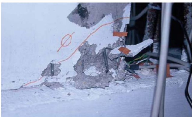
Fig. 9 Experimental damage pattern for T5 motion
