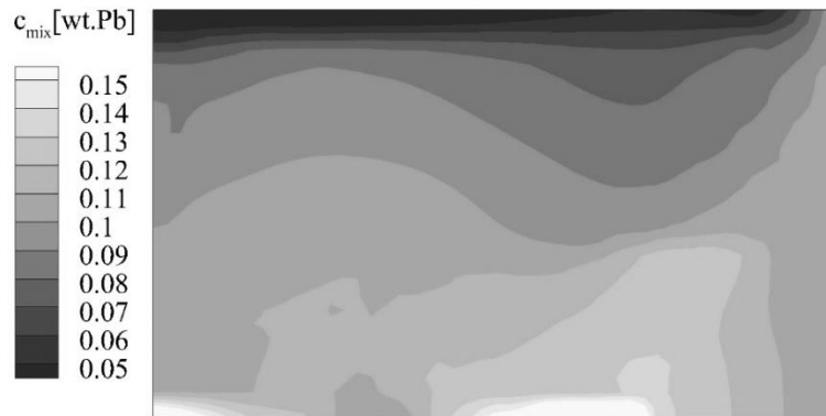
Figure 3. Macrosegregation map obtained from calculation at 1440s.
