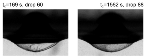
Figure 25. Bending of the hole limit for different coalescence times. Campaign 1, C_{T80} = 0.011 g/L.
