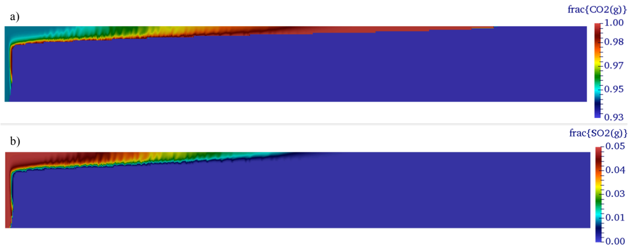
Fig. 7. Injection of 95% CO 2 and 5% SO 2 . Gas composition in mole fraction: a) CO 2(g) and b) SO 2(g) after 30 y of injection. Rescaled zone of reservoir [3000 x 100] m.
