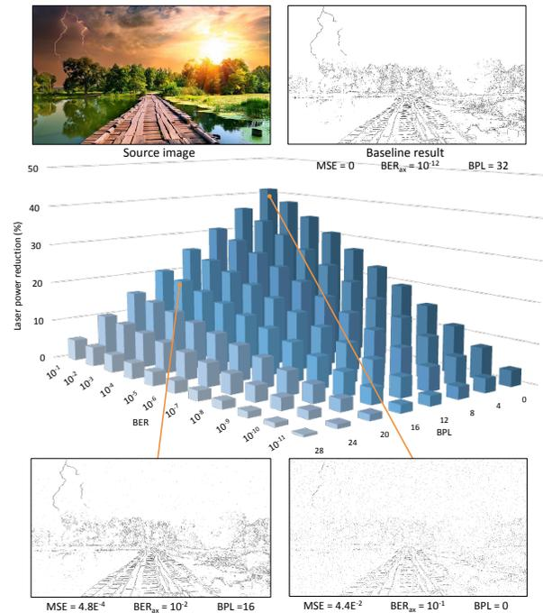
Figure 7: Laser power saving and image degradation for Sobel benchmark application. Results are given for  $BER_{ax}$  ranging from  $10^{-1}$  to  $10^{-11}$  and for BPL ranging from 0 to 28. We assume a 64 cores architecture with 17 clusters,  $N_{data} = 64$ ,  $Ax_{max} = 32$  and  $BER_{not-ax} = 10^{-12}$ .
