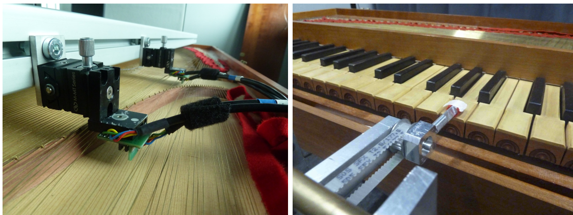
Figure 6. Measurement devices: (left-hand side) optical forks for string displacement. (right-hand side) DRoPi-Crobotic finger for key trajectory control.
