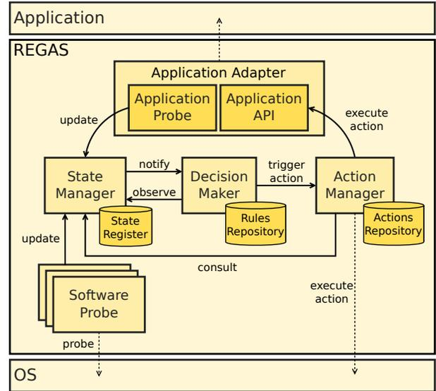
Figure 2. Overall architecture of the REGAS system
