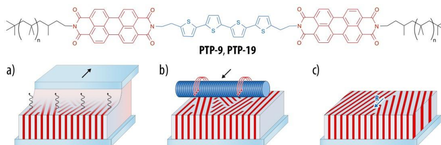
Figure 1. Molecular structure of the polymer-substituted donor-acceptor-donor triads and preparation of thin films. a ) Thin films of PTP-9 or PTP-19 ( n = 9 or 19 , respectively) were prepared by doctor blading and exhibited a lamellar phase with an “edge-on” orientation of the lamellae relative to the substrate and different lateral orientations. b ) Mechanical rubbing and annealing resulted in c ) a macroscopic alignment of the lamellar phase parallel to the rubbing direction.
