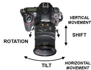
Figure 5: The Nikon D750 DSLR camera with the PC-E Micro NIKKOR 45 mm f/2.8D ED tilt-shift lens used in this paper.
