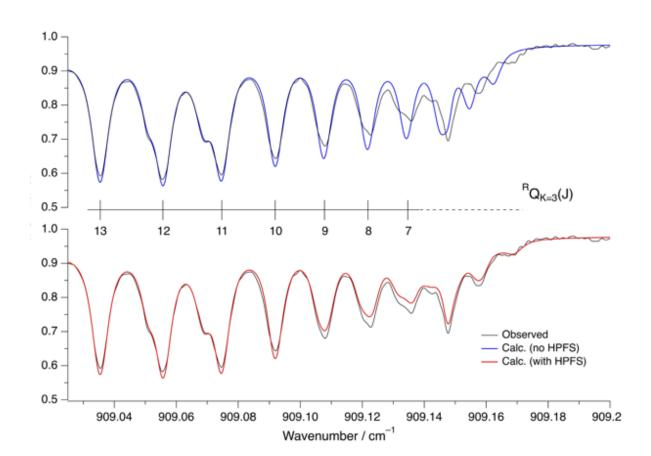
Figure 5  $\label{lem:comparison} \text{Comparison with the Pacific Northwest National Laboratory (PNNL) [16] absorption cross sections in the $\nu_6$ band region (see text for details). }$
